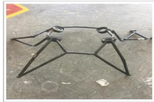
**Fig: Broken Engine mount**
