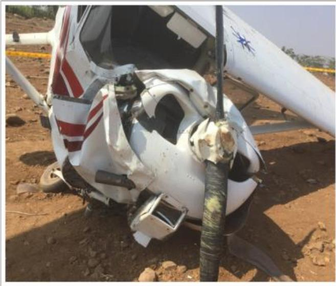
**Fig: Impact on Aircraft Nose**
