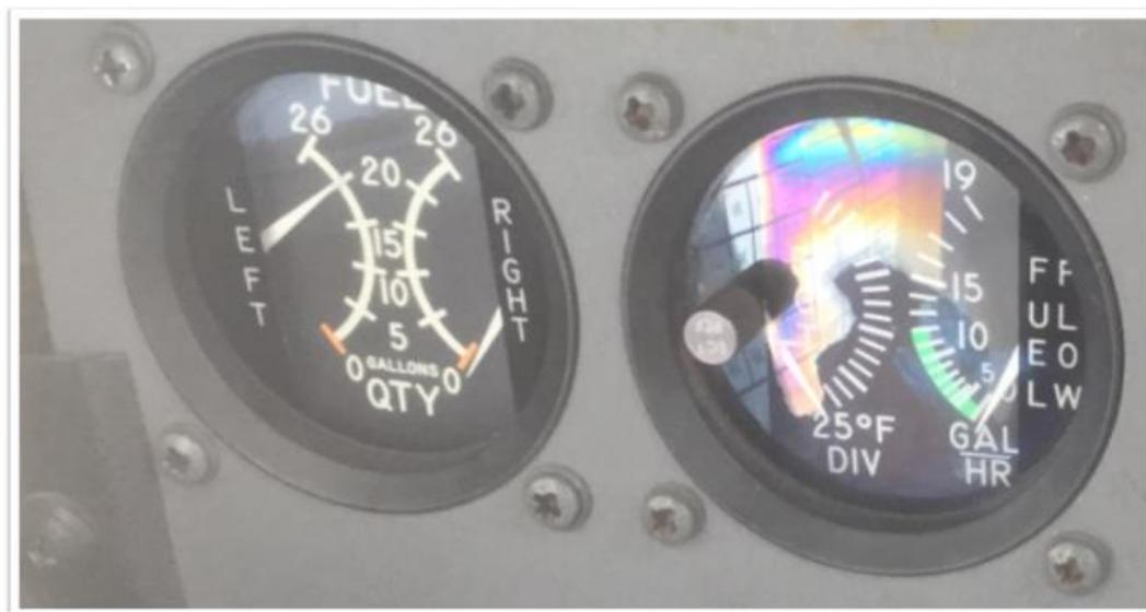
**Fig: Fuel gauges**
